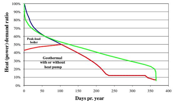
Figure 4. Typical load duration curve for south Iceland (green curve) and central Europe (red and blue curve)
