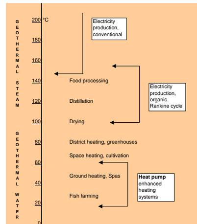
Figure 2 Excerpt from Lándal diagram for geothermal energy
