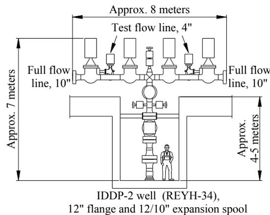
**Figure 3: Well head layout, side view.**
