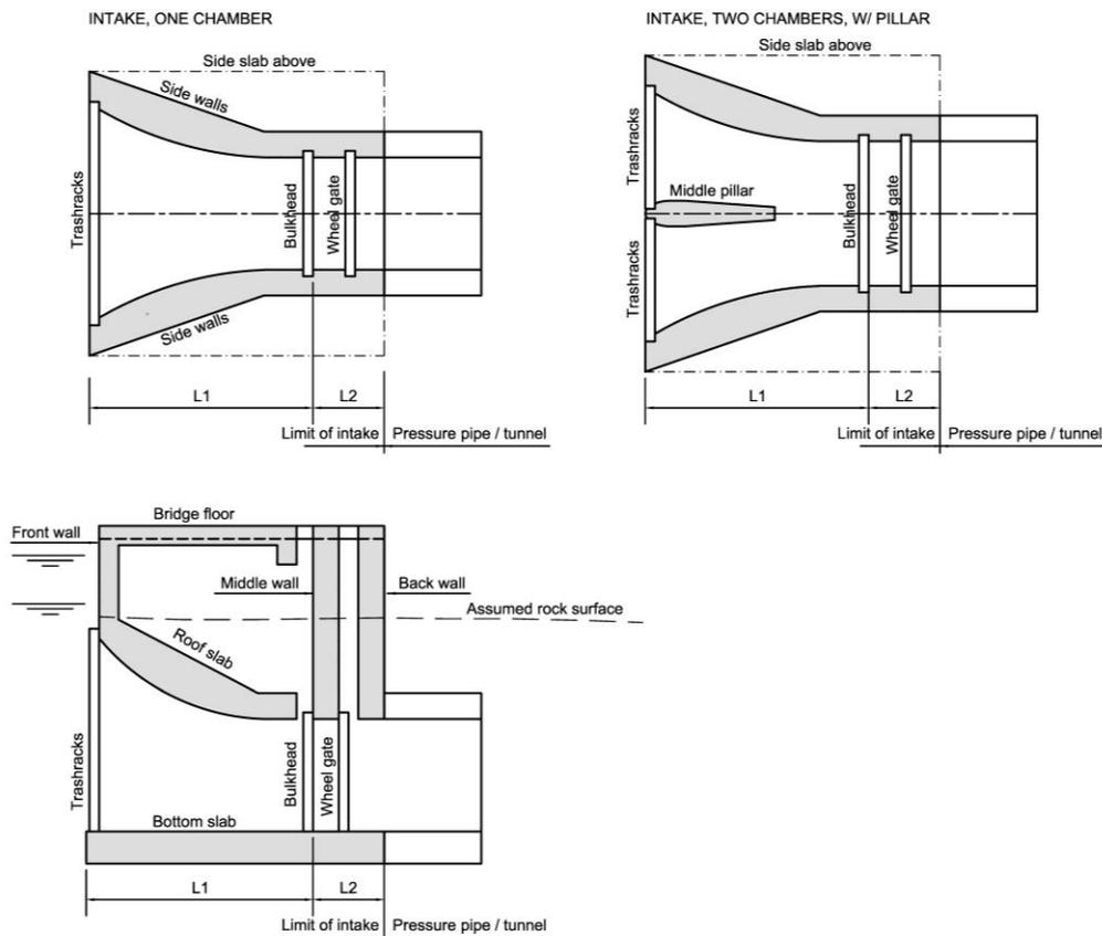
Figure 1. The intake model structure showing the main dimensional parameters (drafted from Gordon (2)).
