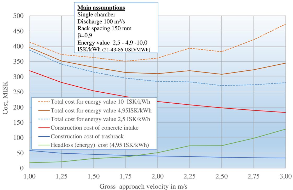
Figure 3. Results of optimisation of trashracks approach velocity with different energy values.
