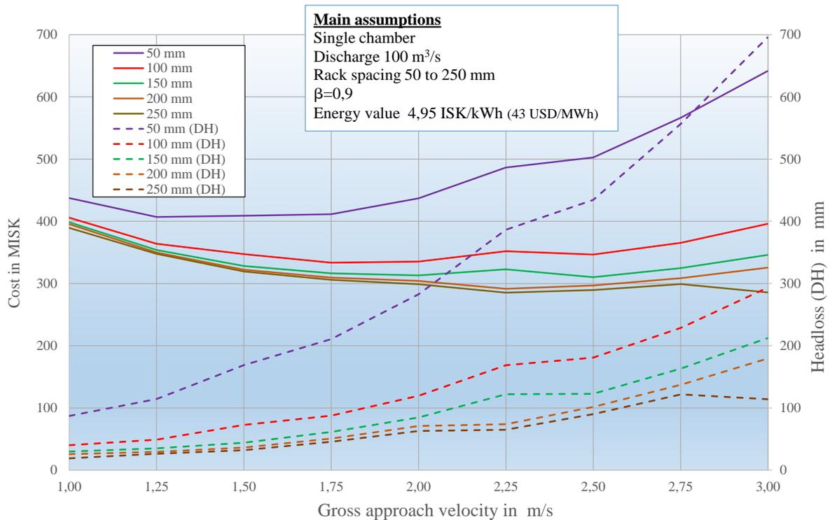
Figure 4. Results of optimisation of trashracks approach velocity for different rack spacing
