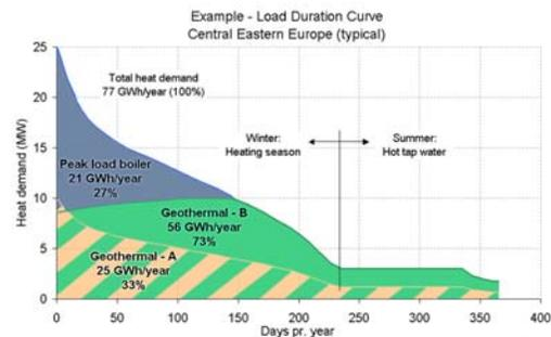
Figure 4. Heat load duration curve – typical for Central and Eastern Europe
