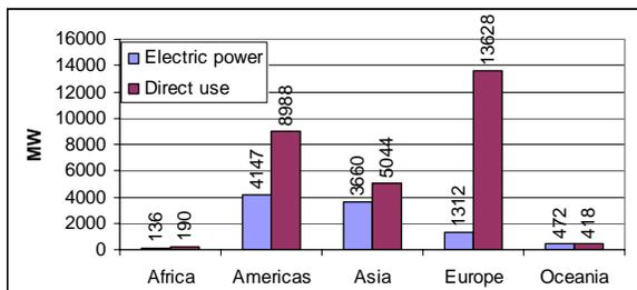
Figure 2. Installed capacity for conventional geothermal electric production and direct use (heating) in different continents in 2007, (adapted from Fridleifsson and Ragnarsson, 2007)
