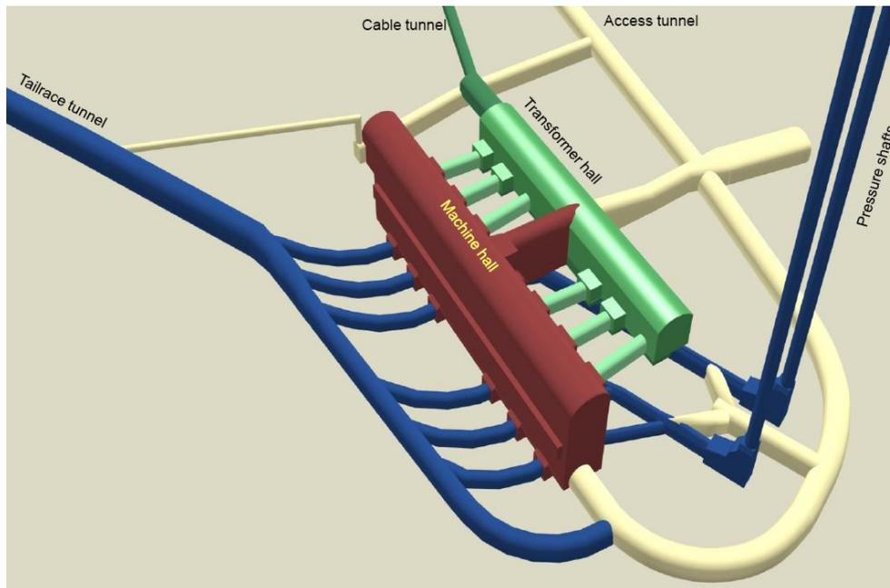
Figure 4. Powerstation perspective view.
