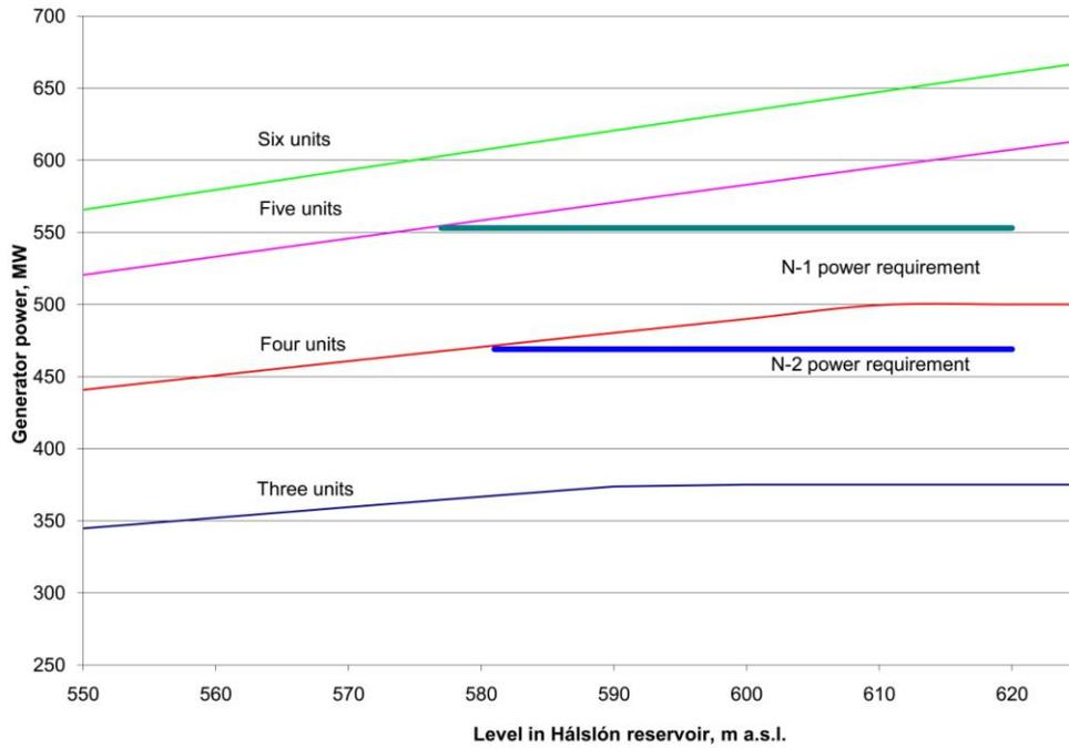
Figure 2. Station power at maximum unit flow.
