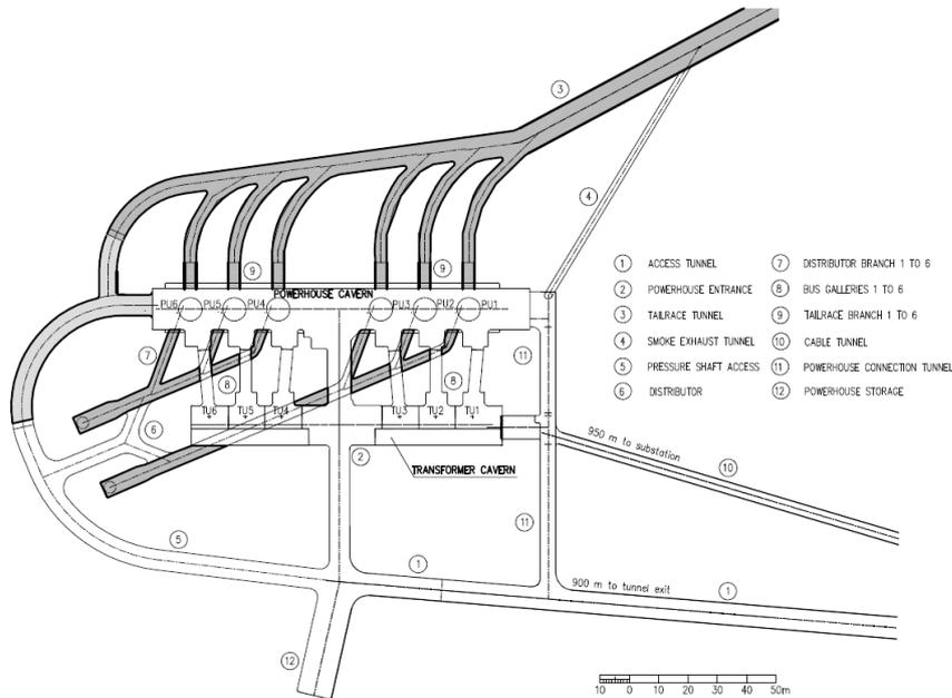
Figure 5. Powerstation plan view.
