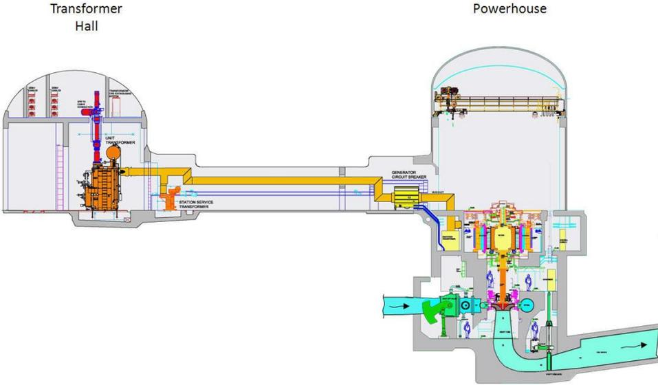
Figure 6. Section through generating unit block.
