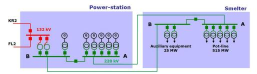
Figure 8. 220 kV system configuration in normal operation.
