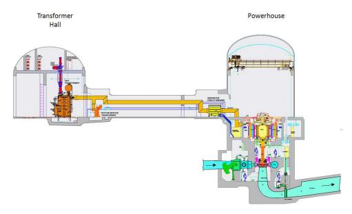
Figure 6. Section through generating unit block.
