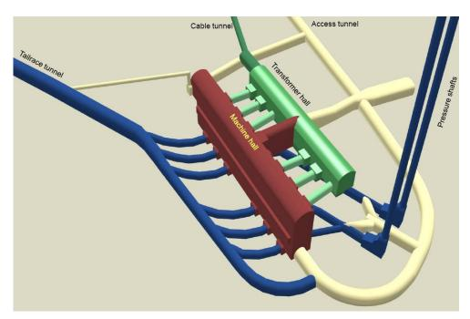
Figure 4. Powerstation perspective view.
