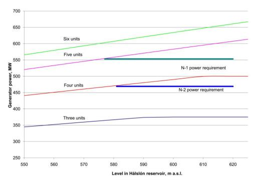
Figure 2. Station power at maximum unit flow.
