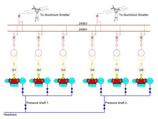
Figure 7. Division of generating units and transmission system.
