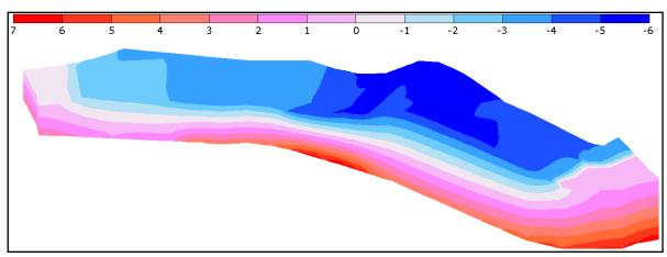
Fig 3 3D-model, isometric view showing temperature profile through rock
