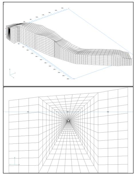
Fig 1 Finite element model, isometric view (above) and cross-section (below)
