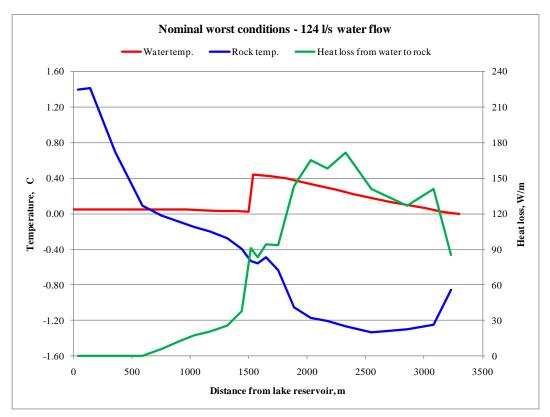
Fig 5 Temperature profile of water and rock by tunnel wall, nominal worst conditions.
