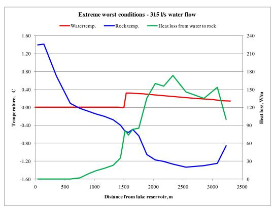
Fig 6 Temperature profile of water and rock by tunnel wall, extreme worst conditions.
