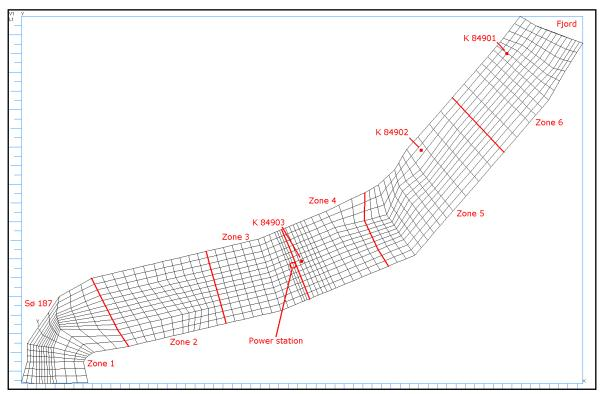
Fig 2 Overview of model zones 1 through 6 and rock temperature measurement boreholes.
