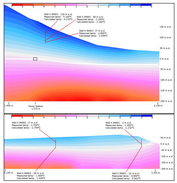
Fig 4 Temperature profile around head- and tailrace tunnel, initial conditions
