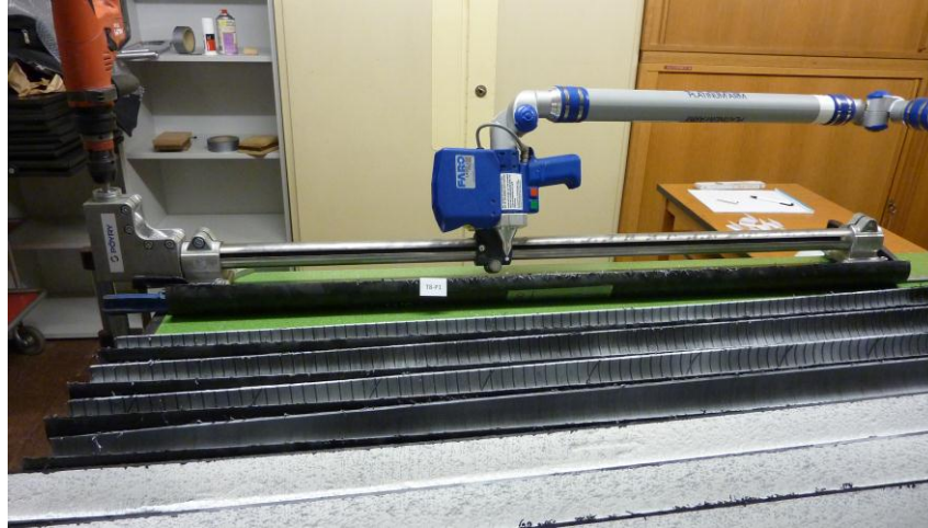
Fig. 4. The laser scan arm scanning the pipes.
