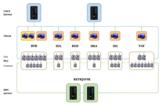
Fig. 3: The network structure of the new Common Area Control System using protocol IEC 60870-5-104
